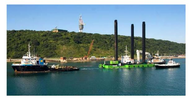
After being reassembled, repaired and lengthened by Elgin Brown & Hamer, the dipper dredger Pinocchio (previously the Toshka) left Durban under tow for a contract in Richards Bay.
